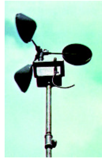
An anemometer - used to measure wind speed
